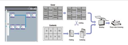
JDF data is automatically output to the post-processing equipment as soon as output of all signatures in a job finishes.
